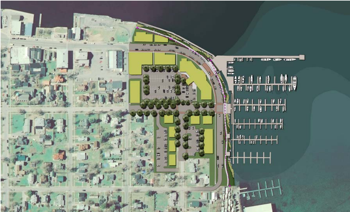
Figure 2: Example build-out plan for the Frink America Property within the Riverwalk C District. Note the plan's integration of the existing street grid pattern and building masses that relate to adjacent properties.
